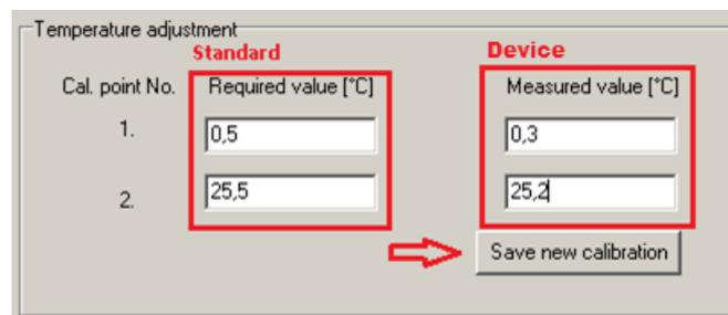
*If the device measured 25.2 °C before adjustment, then after procedure will measure 25.5 °C.*
