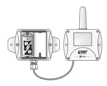
• screw the batteries holder cover. Make sure that the contact surfaces of gasket are free of dirt.
