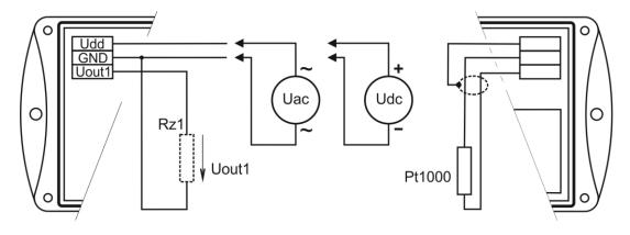
maximum load current of voltage output is 0.5 mA
