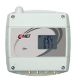
The W0941 sensor with LoRaWAN network output measures temperature from four external Pt1000 probes on the cable. LoRa devices are powered by a replaceable battery with a lifespan of up to 10 years (3 years standard). External power with optional accessories is also available.
