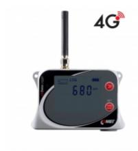
4G datalogger is designed to record CO2 from built-in sensor. In case of exceeded set limits, SMS and JSON messages can be sent via GPRS data connection. Measured values can be sent to the internet storage COMET Cloud, which is a complete monitoring, alarm and analysis system.
