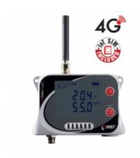
IoT Wireless Datalogger kit with built-in 4G modem and Flat Rate SIM Card allows the instant connection to the COMET Cloud.
