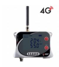
4G datalogger is designed to record temperature and humidity from built-in sensors and temperature from external probe. In case of exceeded set limits, SMS and JSON messages can be sent via 4G data connection. Measured values can be sent to the internet storage <a href="COMET Cloud">COMET Cloud</a>, which is a complete monitoring, alarm and analysis system.
