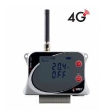
GSM Datalogger is designed to record from two external temperature probes and two two-state inputs. In case of exceeded set limits, SMS and JSON messages can be sent via 4G data connection. Measured values can be sent to the internet storage <a href="COMET Cloud">COMET Cloud</a>, which is a complete monitoring, alarm and analysis system.
