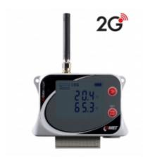
GSM Datalogger is designed to record temperature from four external Pt1000 probes connected to the terminal board. In case of exceeded set limits, SMS and JSON messages can be sent via GPRS data connection. Measured values can be sent to the internet storage <a href="COMET Cloud">COMET Cloud</a>, which is a complete monitoring, alarm and analysis system.
