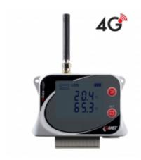
GSM Datalogger is designed to record temperature from four external Pt1000 probes connected to the terminal board. In case of exceeded set limits, SMS and JSON messages can be sent via 4G data connection. Measured values can be sent to the internet storage <a href="COMET Cloud">COMET Cloud</a>, which is a complete monitoring, alarm and analysis system.
