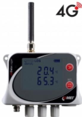
4G Datalogger is designed to record temperature from four external Pt1000 probes. In case of exceeded set limits, SMS and JSON messages can be sent via 4G data connection. Measured values can be sent to the internet storage [COMET Cloud](#), which is a complete monitoring, alarm and analysis system.
