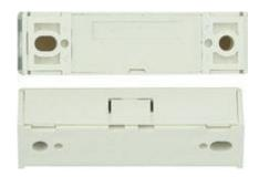
Magnetic door contact, connectable to binary inputs, without cable. Plastic body, the cable wires are connected to terminals inside the housing. The dimensions of 49x14x13mm, working distance of 30 mm.
