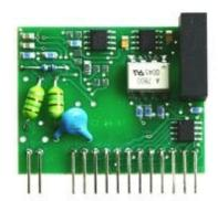
Accuracy  $\pm 0.1\%$  FS. Galvanic isolation is not designed as safety protection.
