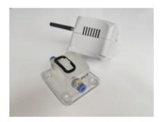
Accessory is designed to verify the measuring accuracy (calibration) and new adjustment of instruments sensing the air relative humidity.
