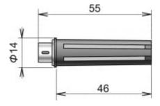
Digital probe with connector MiniDIN, for direct insertion.
