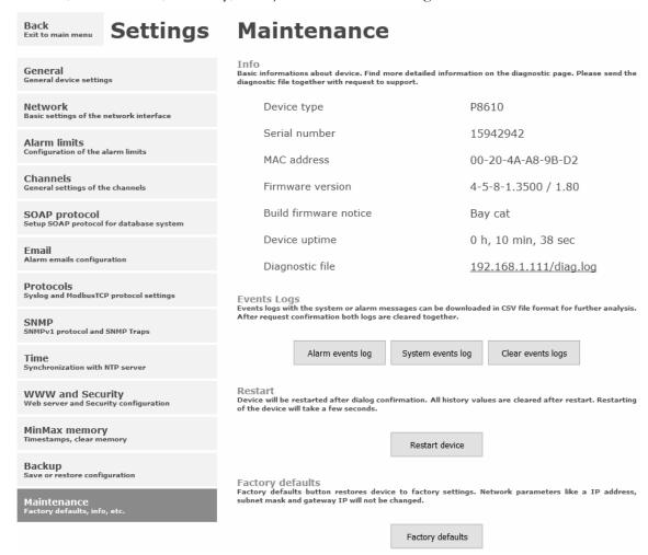
Network parameters are changed while you press button at left side of device during power supply connection. Factory defaults have no effect to user correction inside probe.
