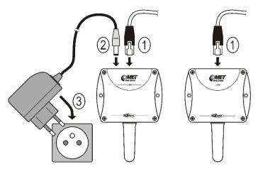
Web Sensor P8611 and P8641 connection (power supply adapter, Power over Ethernet):
