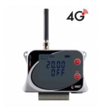
GSM datalogger is designed to record 3 current inputs and 1 binary input. In case of exceeded set limits, SMS and JSON messages can be sent via 4G data connection. Measured values can be sent to the internet storage COMET Cloud, which is a complete monitoring, alarm and analysis system.
