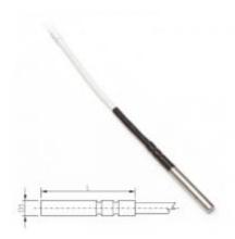
Multi-purpose watertight IP67 probe -190 to +150°C. Accuracy class B. Stainless steel 17240 with teflon cable of specified length, with CINCH connector. Diameter  $5\pm0.1$  mm, length 50mm.
