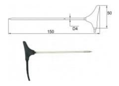
Temperature probe with Pt1000 sensor.
